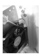
4. Remove (4) screws from the fan mounting bracket.
